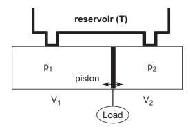
Fig. 3. Work extraction by a movable piston separating two chambers (e.g., of an ideal gas) of fixed overall volume  $V^1 + V^2 \equiv V$ . The piston is connected to a load, allowing it to maintain differential pressures  $p^1$  and  $p^2$  in the two chambers while trading volume between them, equivalent to differential prices under exchange of commodities. A reservoir at temperature T permits reversible transformations while the other variable V is conserved.
