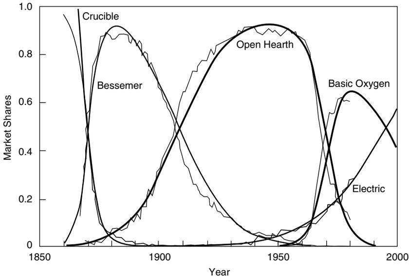
**FIGURE 7** Process technology change in US steel manufacturing, in fractional shares of raw steel tonnage produced. SOURCE: Nakićenović (1987).
