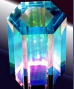
High optical quality ultrahigh vacuum compatible hexagonal cell for neutral atom quantum computing developed under IARPA MQCO program.
