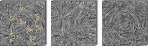
Fig. 5. Two-dimensional results provided by Tong et al. [97]. L-R: The original field, \vec{\xi} , irrotational ( \vec{d} ), and incompressible ( \vec{r} ) components. The divergence and rotation in critical points in \vec{\xi} are shown in yellow.
