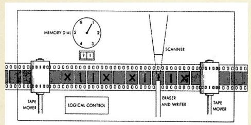
A Turing machine . T = (S, A,  $\delta$ , s0, b, F) consists of: . S = a finite set of states . A = an alphabet .  $\delta$  : Sx(A U {b})  $\rightarrow$  Sx(A U {b})x{L, R}, the transition function,
