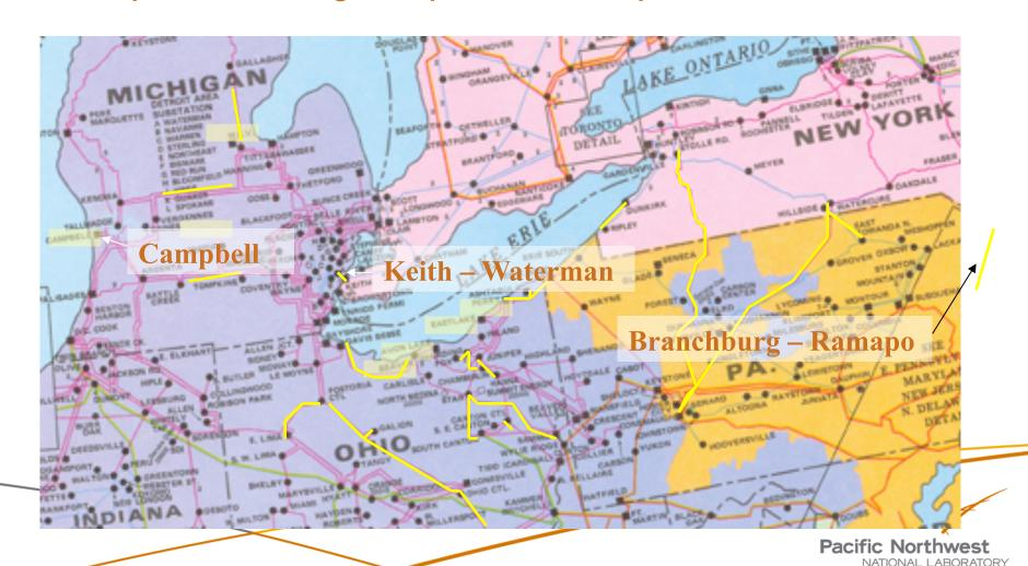
After the Branchburg – Ramapo 500 kV line trips, the underlying 230 kV and 138 kV ties in New Jersey trip, leaving northern New Jersey connected with New York, and southern New Jersey and Pennsylvania remain connected with the remainder of the eastern Interconnection.
