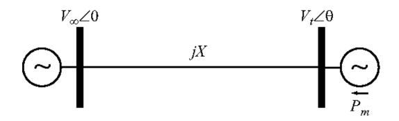
For a single machine infinite bus system, the swing equation becomes:
