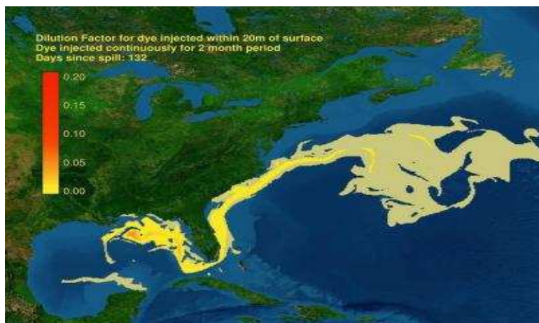
Figure 1: A snapshot at day 130 from a dynamic simulation showing how oil released at the location of the Deepwater Horizon disaster in the Gulf of Mexico would spread. ( http://www2.ucar.edu/news/2154/ocean-currents-likely-carry-oil-along-atlantic-coast 08/23/2011)
