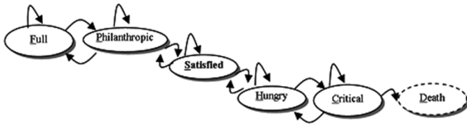
Fig. 4. Agent state transition diagram. Note that additional state transitions are possible directly between full, philanthropic, satisfied, hungry, and critical states, but the ones shown are the most frequent.
