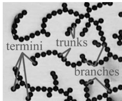
Fig. 3. Detail of the final network from Fig. 1f. The network is characterized by the three types of particles shown in the figure. Termini touch only one other particle; trunk particles touch exactly two other particles; and branching points touch three or more particles.
