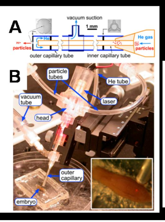
Pneumatic Capillary Gun for Biolistic Intracellular Delivery of Molecular Reagents
